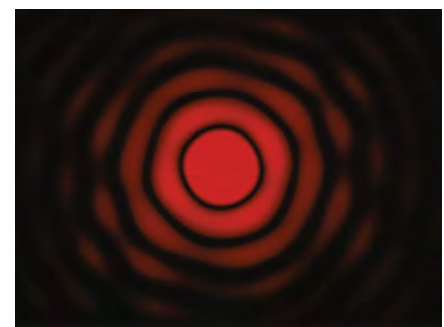
Figure 3.51 The interference pattern created when light diffracts through a circular aperture rather than a single slit.
