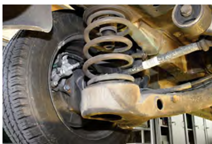
Figure 2.5 Vehicle suspensions can act like mass–spring systems.
