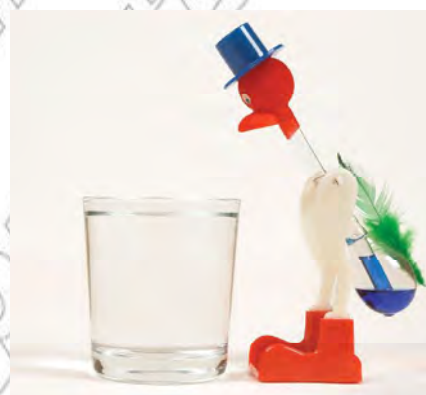
Figure 1.26 The drinking bird is an example of a heat engine; the temperature difference between the room and the cooler water drives the bird.
