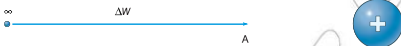
Figure 4.35 The electric potential at A is equal to the work done per unit charge in moving a positive test charge from infinity (i.e. a long way away) to point A.
